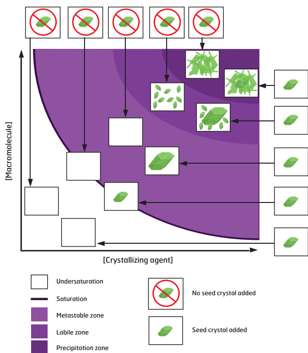
Figure 1: Seeding and the phase diagram. From Luft and DeTitta, Acta Cryst. (1999) D55, 988–993.
